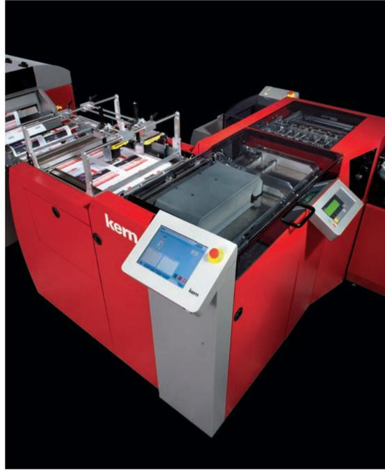
**Kern Continuous Forms Cutter Sigr/L with Integrated Grouping and Folding Station**
